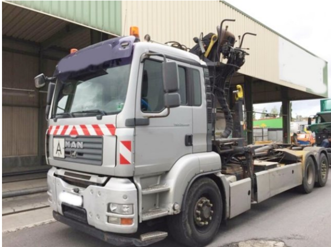
MAN TGA 26.44.0 6x4H-2 BL, HydroDrive, Kran Epsilon E120Z79, Liftachse
